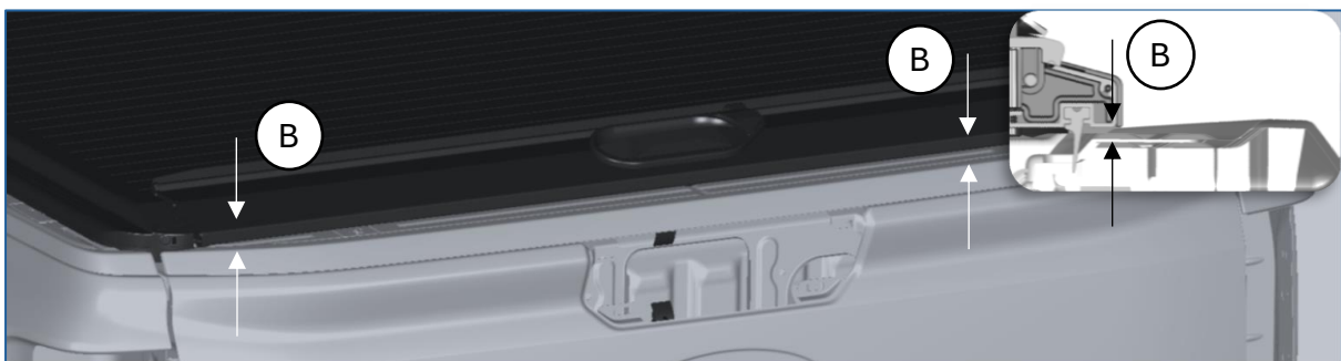
Figure.7 – Adjust the two rear brackets up or down until the gap between the rear profile and the top of the tailgate surface is 10mm.
