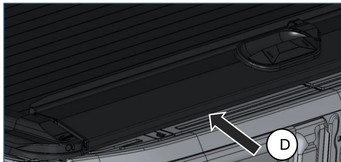
Figure.25 – Ensure that the rubber tailgate seal is forming a sealing along the full length of the tailgate. Excessive squish between the seal and the load bin may result in a poor seal join.
